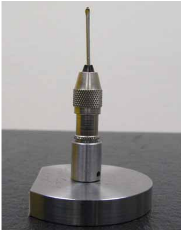
Figure 2-3 Sample Holder – Pin Vise with Sample on Thin Rod
