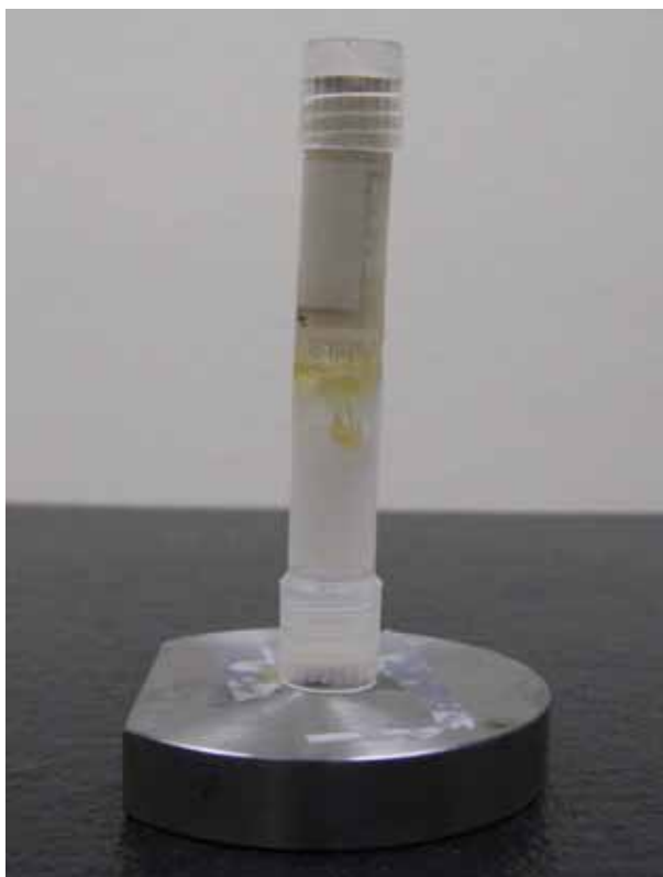
Figure 2-4 Sample Holder – Sample Base with Sample in Plastic Tube
